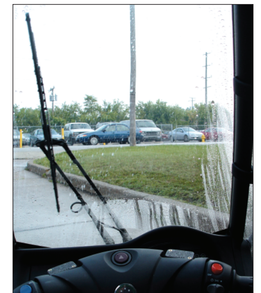
Award-winning Quantum coating is used in many tough applications. Our Quantum coated polycarbonate has withstood over one million windshield wipes on the windshield of the fully enclosed Benelli Adiva scooter.
