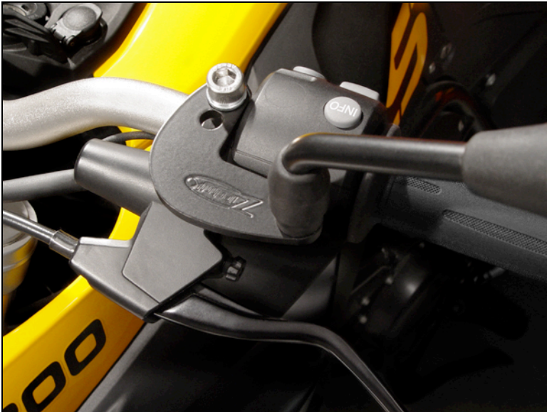
The Z5301 is contoured to fit tightly against the F800GS control housing while not interfering with the power switch!
